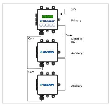
The optional wired Primary Controller can be purchased with any TDP05K system. All probes become Ancillary, and the separate wired Primary Controller can be mounted up to 500 feet from the TDP05K ancillary probes.
